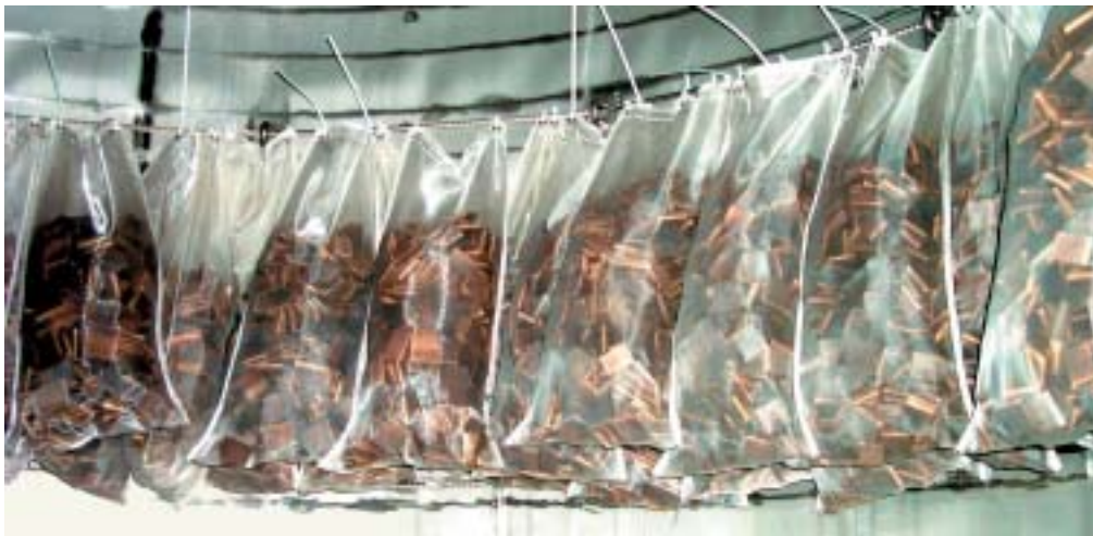
Segment bags tied to stainless cable inside 20,000 gallon tank.
